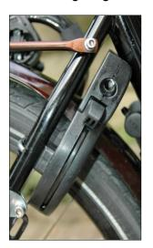
LOCKER: As we also use our tandem in the city, we have fitted it with a locker on the frame. Since the space available for this type of locker is very limited, we have opted for the Trelock RS400 with a V punch
