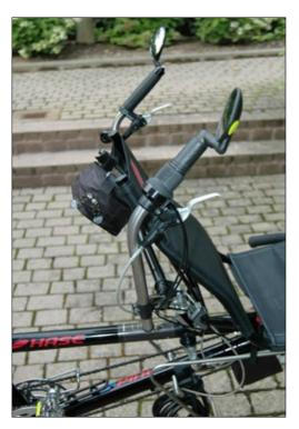
Handles' position. As mentioned above, the original position, with an angle of approximately 100° is uncomfortable. We asked to fit a handlebar with a 130° angle and the result exceeds all our expectations, to the extent that "Swiss Fun Rent" plans to equip its rental Pinos with such handlebars. This way, the rotating Rolhoff and SRAM handles can remain in their normal position.
